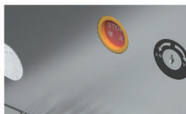
急停按钮 Emergency Stop Button
